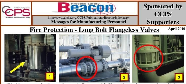
Would you recognize the metal cover (yellow arrow) in Picture 1 as an important piece of safety equipment? If it was damaged or missing, would you know to report it so that it could be repaired or replaced?
