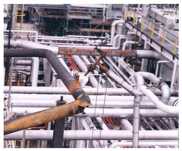
Figure 9 – In-situ failed elbow and injection pipework connection (broken off)
