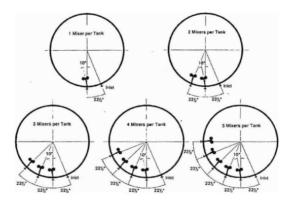
Appendix 2 Recommended Mixer (Swivel-Angle) Positions for Effective B.S. And W Control In Crude Oil Tanks
